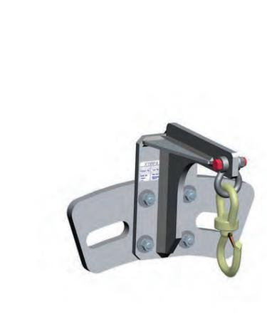
Used for vertical or horizontal accesses with pole hoist systems. Can be installed on a round or square inlet flange with strength capacity of at least 22 kN. Connector included.
