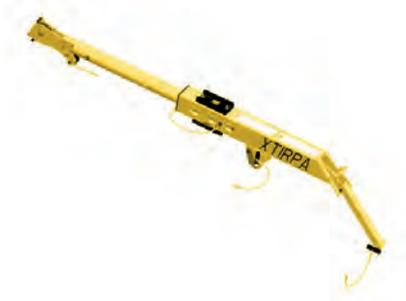
Equipped with retractable system and winch bracket to ease access in confined spaces. To be used with mast art. **IN-2003** and an appropriate base or with self-supporting manhole guard art. **IN-2108**. Extensible form 1431 to 1884 mm. Equipped with a 22 kN anchor point.
