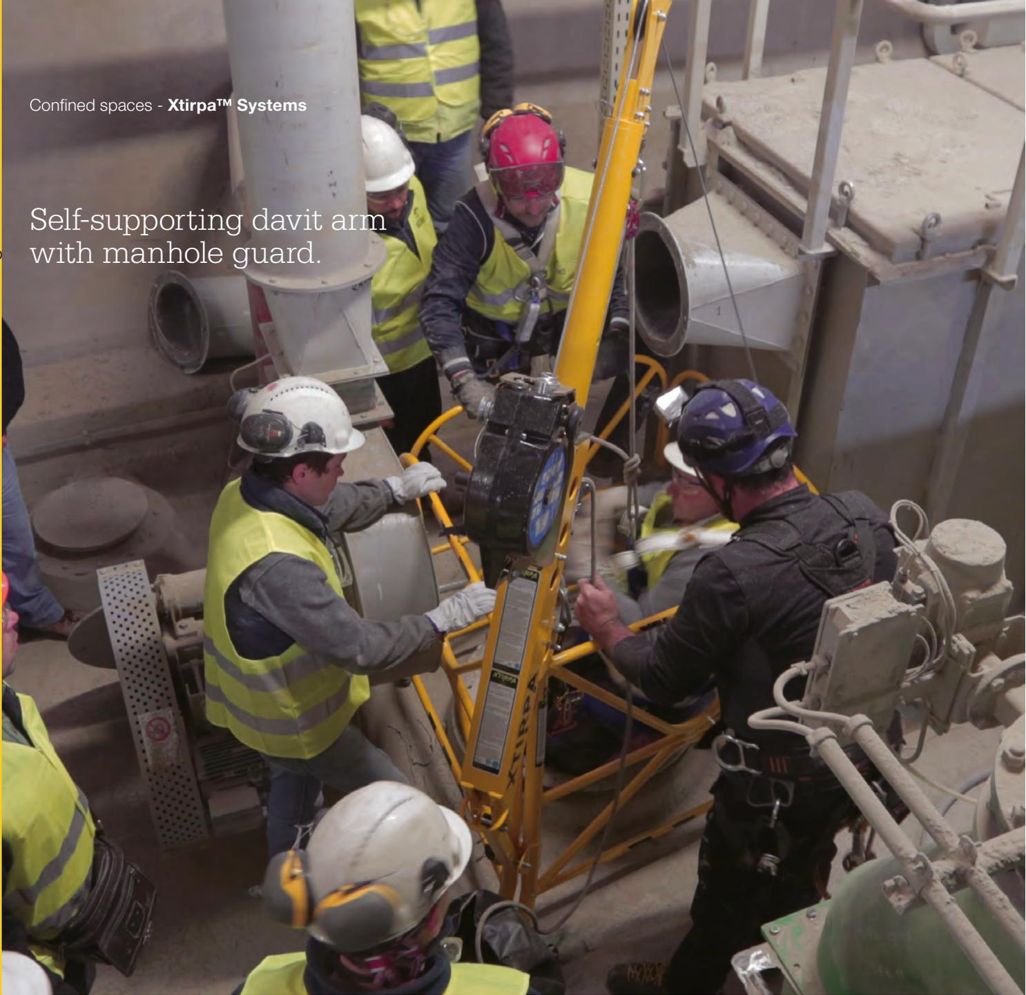
Used when access requires railing protection and a base can't be installed.
