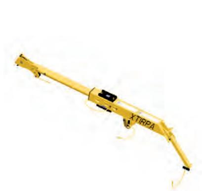
Equipped with retractable system and winch bracket to ease access in confined spaces. To be used with mast art. **IN-2003** and an appropriate base or with self-supporting manhole guard art. **IN-2108**. Extensible form 1431 to 1884 mm. Equipped with a 22 kN anchor point.
