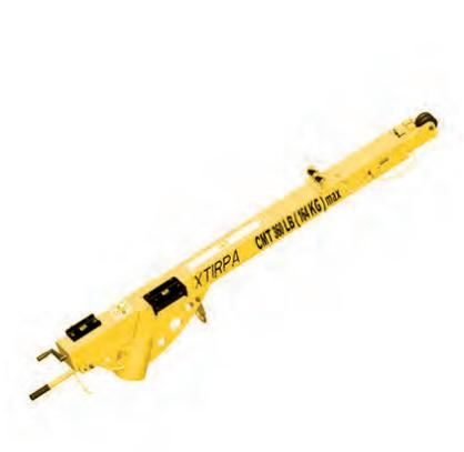
Equipped with retractable system and winch bracket to ease access in confined spaces. To be used with mast art. **IN-2199** and an appropriate base. Extensible from 2493 to 3497 mm. Equipped with a 22 kN anchor point.
