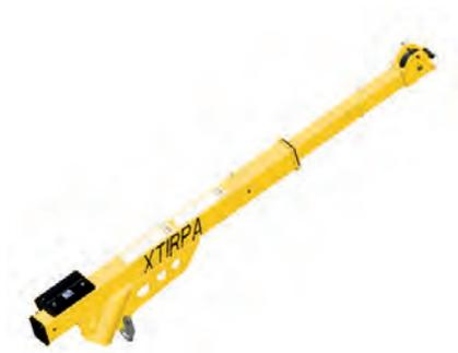
Equipped with retractable system and winch bracket to ease access in confined spaces. To be used with mast art. **IN-2240**. Extensible form 1422 to 1965 mm. Equipped with a 22 kN anchor point. Optional winch attachment (art. **A2237-06**).
