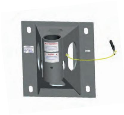
Spaces out the mast from the wall by 200 mm to allow davit arm movement. Bolts not included. Also available with 350 mm distance (art. **IN-2067**).
