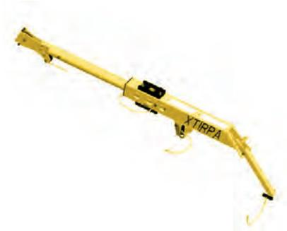
Equipped with retractable system and winch bracket to ease access in confined spaces. To be used with mast art. **IN-2003** and an appropriate base or with self-supporting manhole guard art. **IN-2108**. Extensible form 1431 to 1884 mm. Equipped with a 22 kN anchor point.
