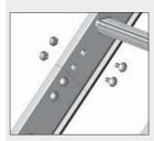
Connect the roof ladders using the connecting straps, Ref. No. 1049.x03. The bolts, washers and locking nuts are included. Use four bolts per strap. At least two safety hooks must be used. Up to three ladders can be joined without an additional roof hook and fastening bracket being needed.
