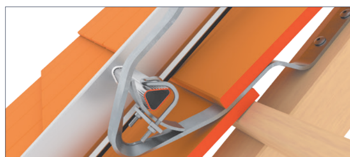
Exemplary application of the safety hook model Z (Pos. 1)
